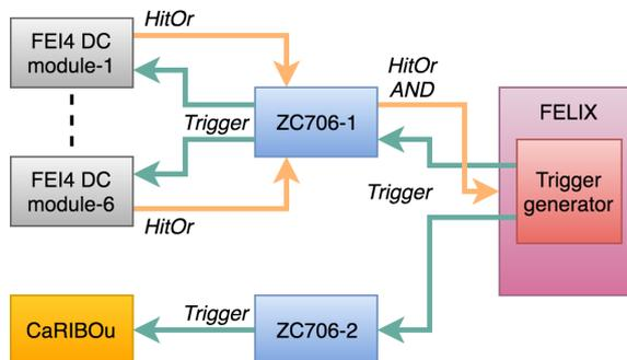
**Figure 16.** Trigger flow in testbeam.
