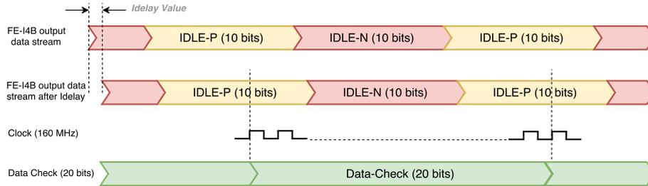
**Figure 11.** FE-I4B output data phase calibration.
