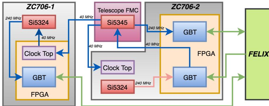
**Figure 10.** Clock distribution in the front-end electronics.
