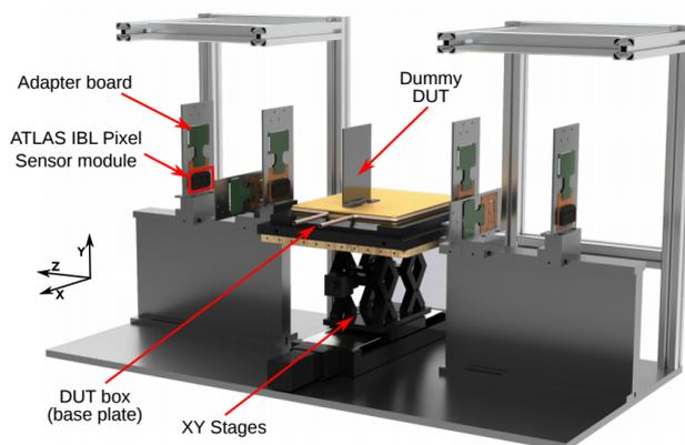
**Figure 2.** Computer generated image of the testbeam Telescope setup. Reproduced from [5]. © 2016 IOP Publishing Ltd and Sissa Medialab srl.
