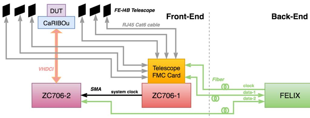
**Figure 5.** Test setup of testbeam Telescope and CaRIBOu readout with the FELIX.
