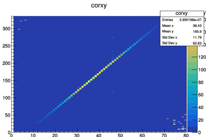
**Figure 19.** XY correlation of two FE-I4B telescope planes.
